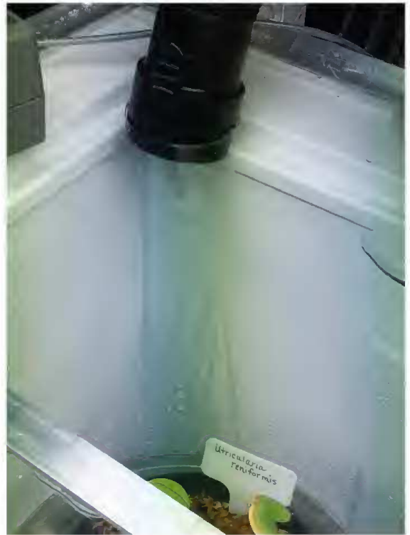
Figure 2: Shop vac hose from the humidifier, placed through a hole drilled through the lid, for added humidity.
